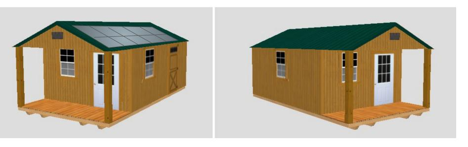
12' x 24' Office and Food Pantry with 12' x 20' interior (4' front porch) Front entry and counter for customer interaction Side and rear entry for food donation collection and organization Solar (~4kW) on south facing roof with electric baseboard heat
